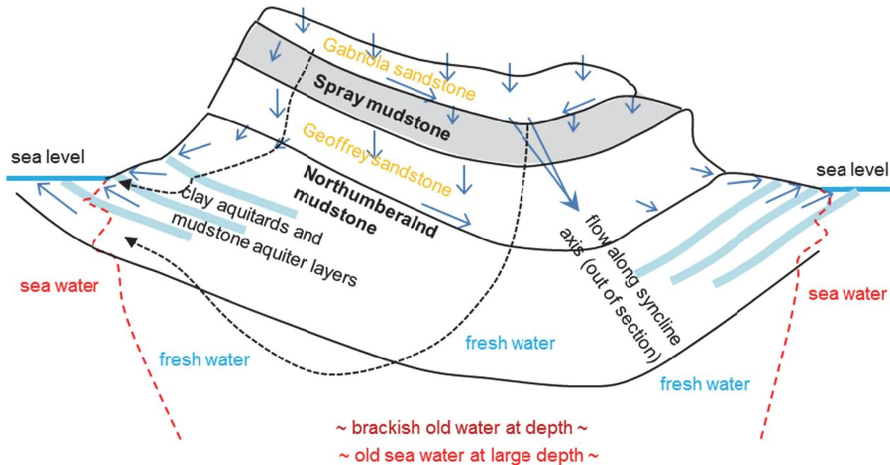
**Figure 10: Groundwater flow in conceptual model of Gabriola Island.**
