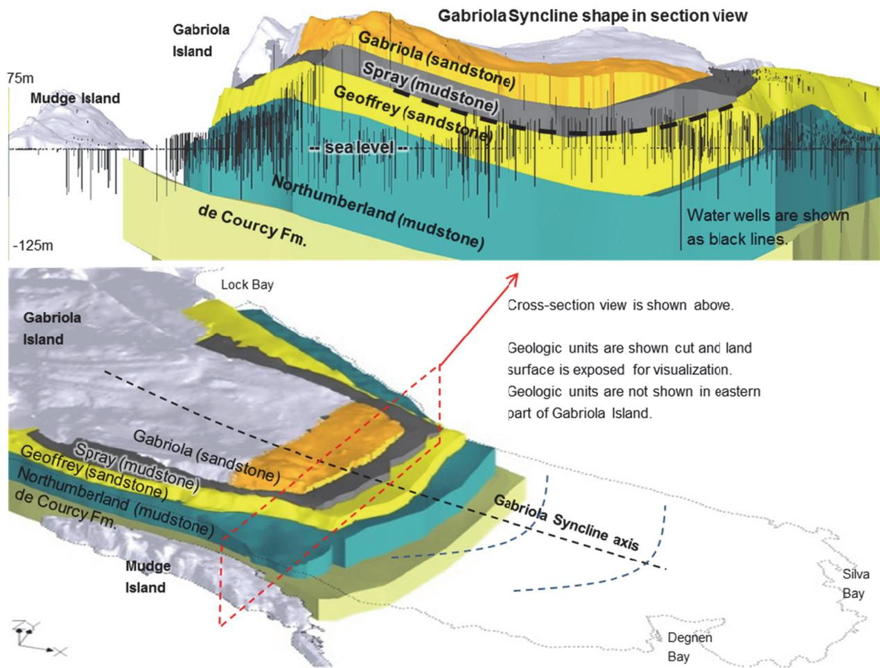
**Figure 3: Gabriola syncline and geological units in cross-sections.**
