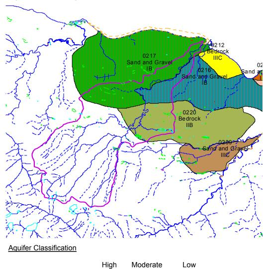
Figure 1 Developed groundwater aquifers in the French Creek area
