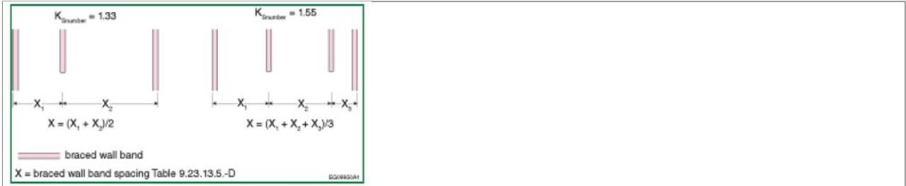
Figure A-9.23.13.7(4)-C Calculation of Mean Braced Wall Band Spacing for Seismic When the Spacings between Adjacent Braced Wall Bands are Not Uniform
