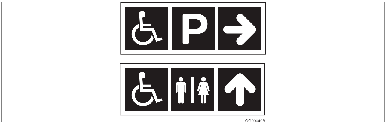
Figure A-3.8.3.9.(3)-A Signs indicating accessible facilities
