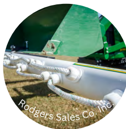
Wick applicator attached on a tractor
