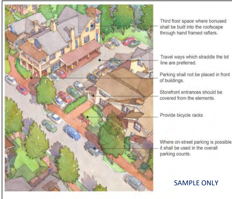
Example of desirable design elements such as mixed on and off-street parking and shared travel ways between developments.
