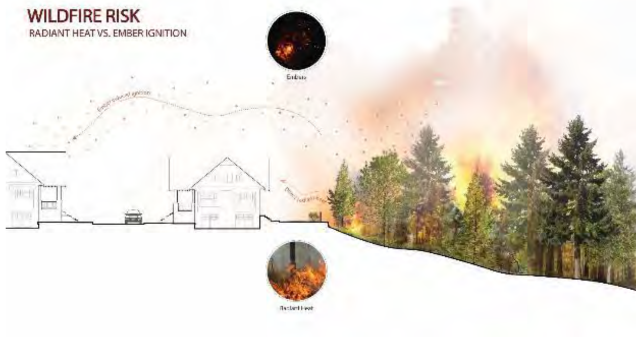
Figure 15. Pathways to home ignition in the WUI.
