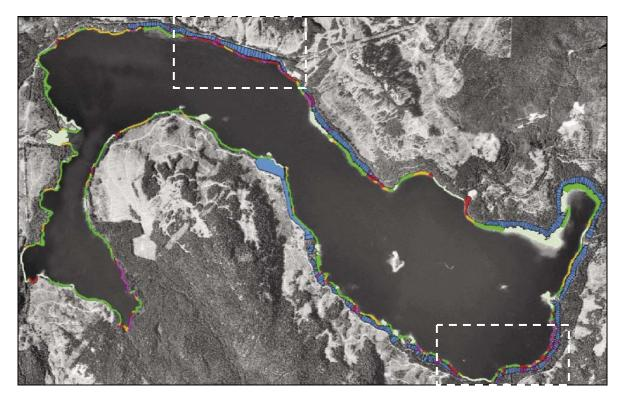
Figure 11 – Horne Lake Erosion Assessment results. Areas of red and purple have been designated as high and very high erosion hazard respectively, with blue representing lot coverage (*Source: Guthrie and Law, 2005*)
