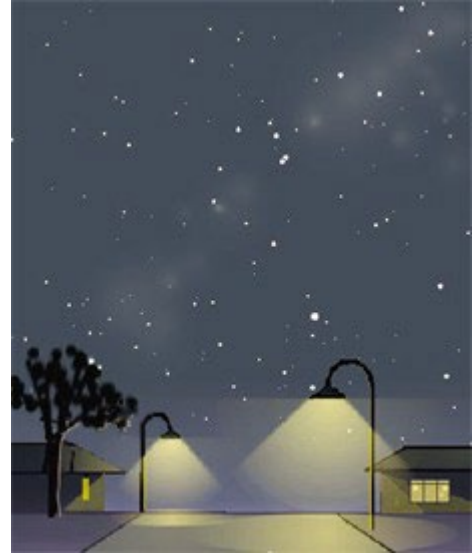
Example of full cut-off light fixtures with direct light below the horizontal plane reducing light pollution and protecting the night sky.
