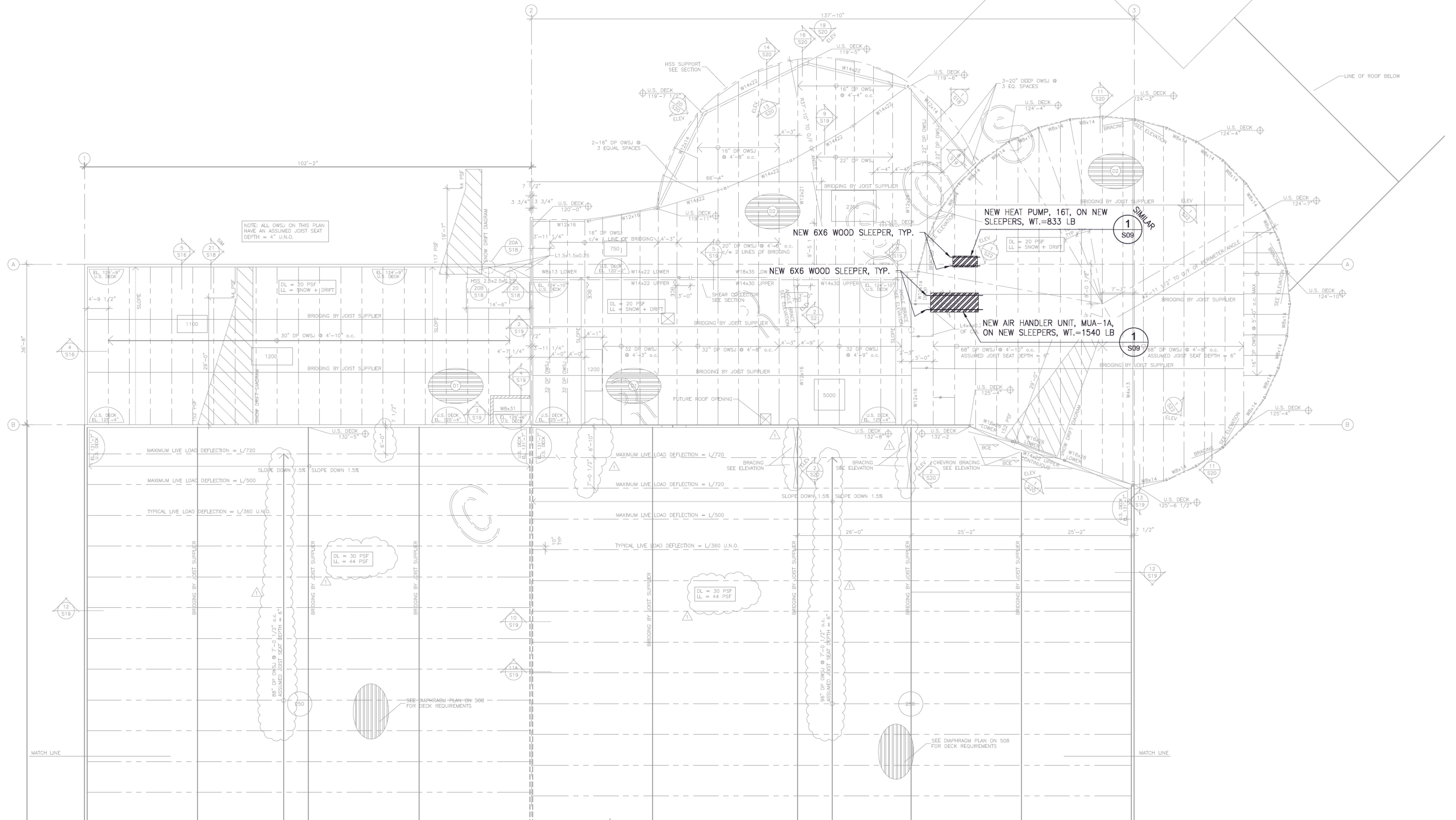
EAST ARENA UPPER ROOF FRAMING PLAN 3/32" = 1'-0"
