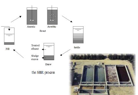
Figure 2 Sequencing Batch Reactor Process
