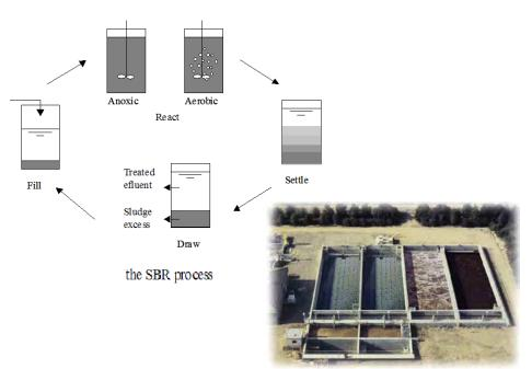
There are several variations of the SBR process. One of the more common variants is the Intermittent Cycle Extended Aeration System. The Intermittent Cycle Extended Aeration System has a small pre-react chamber at the influent end of the SBR tank and a baffle wall
