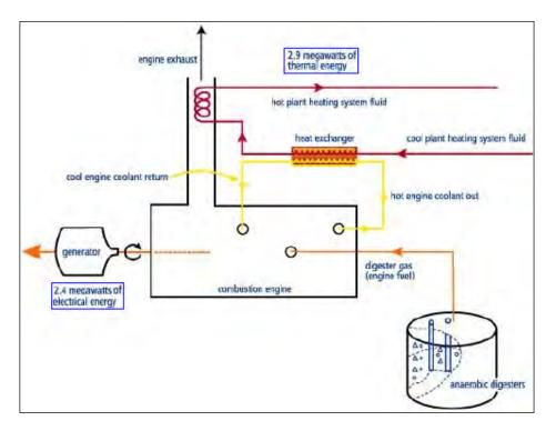
Figure 2. Typical Wastewater Treatment Plant Co-Generation Facility
