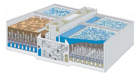
BAFs typically have relatively short sludge ages (SRT) and as such, are similar to trickling filters in their relatively poor capabilities of removing EDCs and PPCPs.
