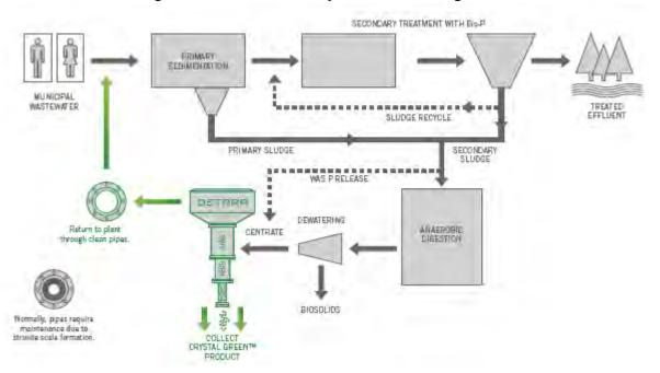
Figure 3. Nutrient Recovery and Struvite Mitigation
