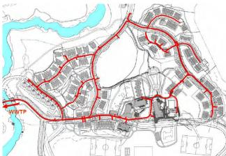
Heat exchangers at the WWTP will transfer the heat contained in the effluent to water contained in the DHS closed loop piping network. The addition of the heat exchangers to the WWTP comes at the convenient time when the plant is undergoing a major capacity upgrade. The pipe network will extend more than a kilometre from the plant to and across the village.
