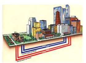
Low temperature networks are best for cases in which the pipeline must extend more than one kilometre from the utility to the customers. The temperature of the water that circulates from the utility to the user ranges usually from 10 to 20°C. According to SuisseEnergie, less expensive non-insulated pipes can be used since heat losses to the ground are small because of the small temperature difference between the ground and the water in the pipe.
