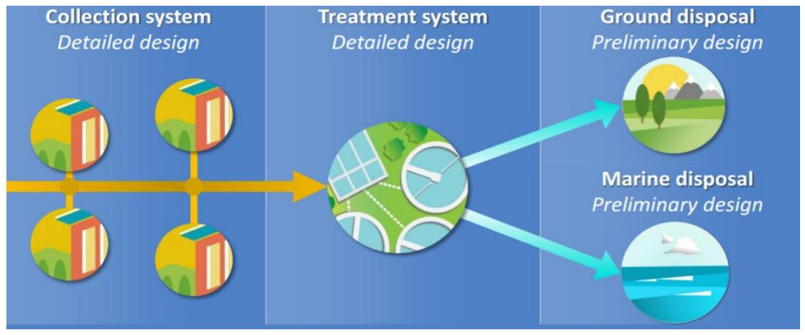
• The sewer systems can be broken into three major components – Collection System, Wastewater Treatment Plant (WWTP), and Outfall.
