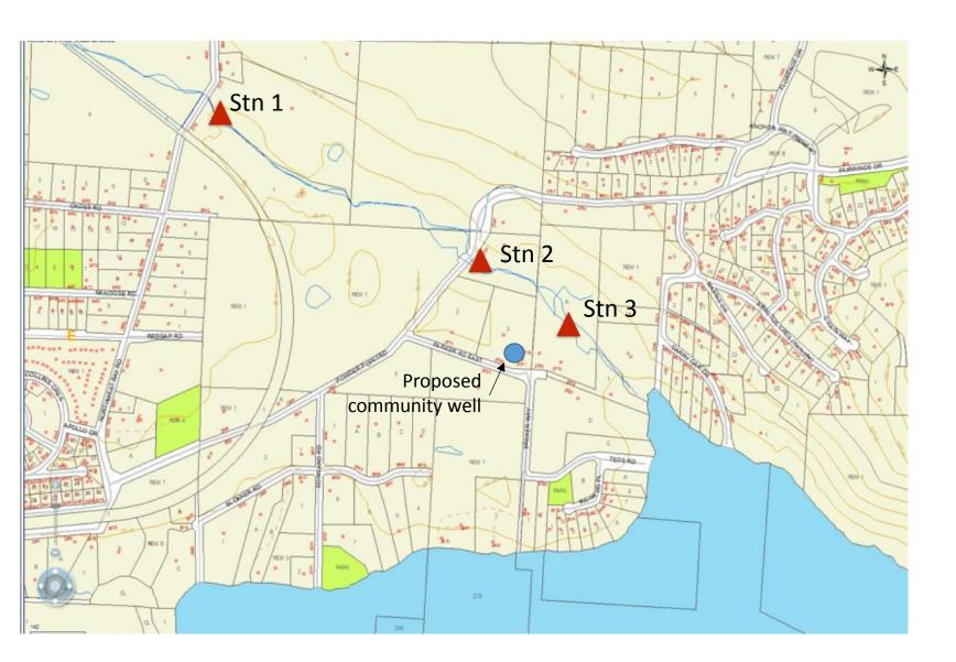
To evaluate connection with aquifers - river base flow is a criteria for sustainable operation of a well
