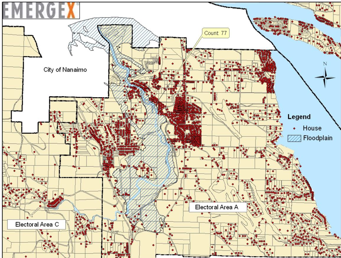
**Figure 12 – Houses contained within the Nanaimo River floodplain in Electoral Area A**
