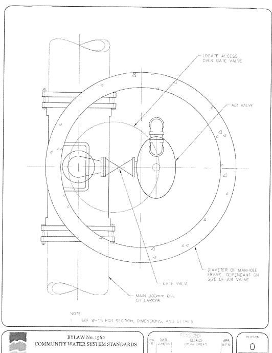
AIR VALVE 75mm DIA. AND LARGER PLAN
