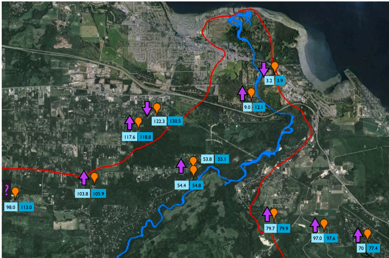
Figure 12: High and low water levels recorded in 2013-2014 and direction of vertical groundwater movement in purple arrows
