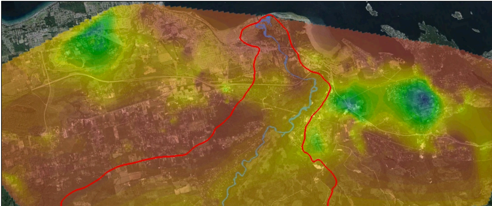
Figure 6: Map of depth to bedrock with blue/green shading being deep points and yellow/reds shallower
