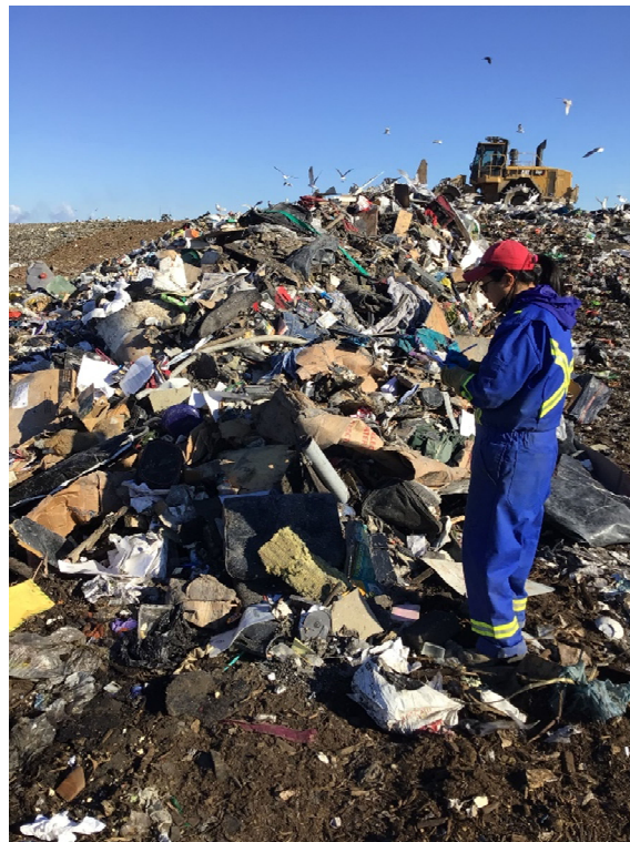
Photo 6: Field Staff Conducting a Visual Estimate of a Tipped Load
