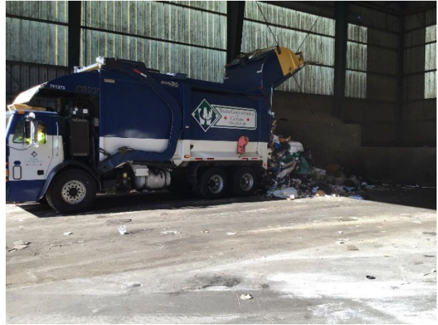
Figure 2-4: Front-load Truck Tipping an ICI Load at the CRTS
