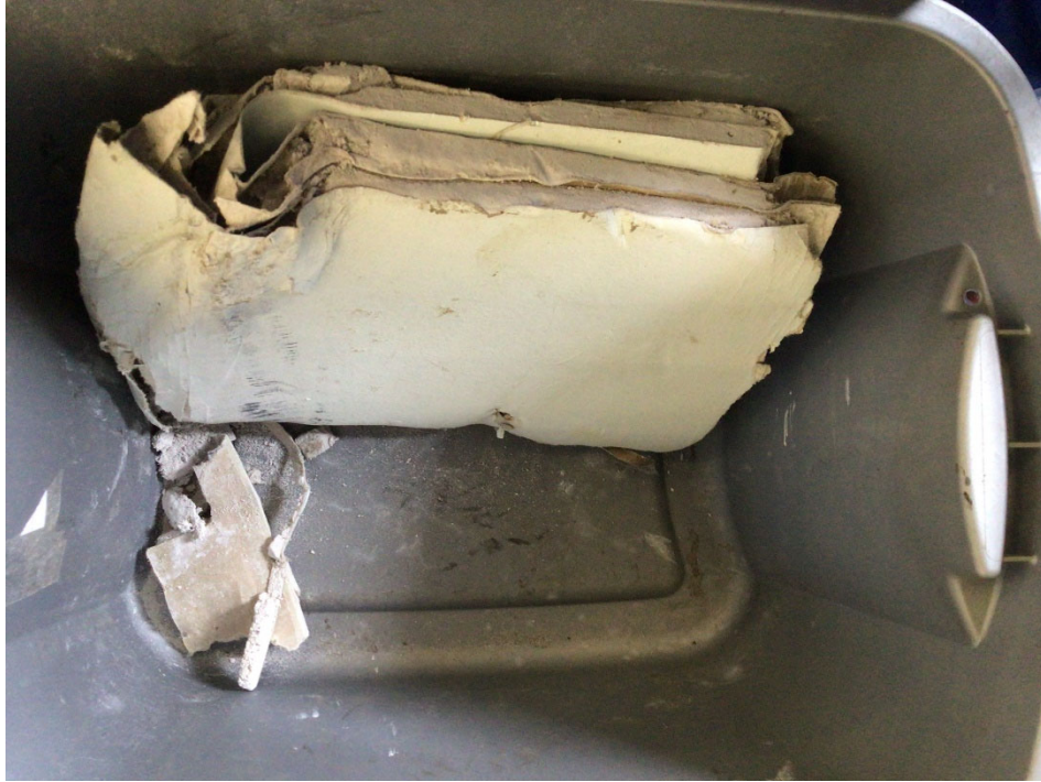
Photo 27: Example of the Drywall Category
