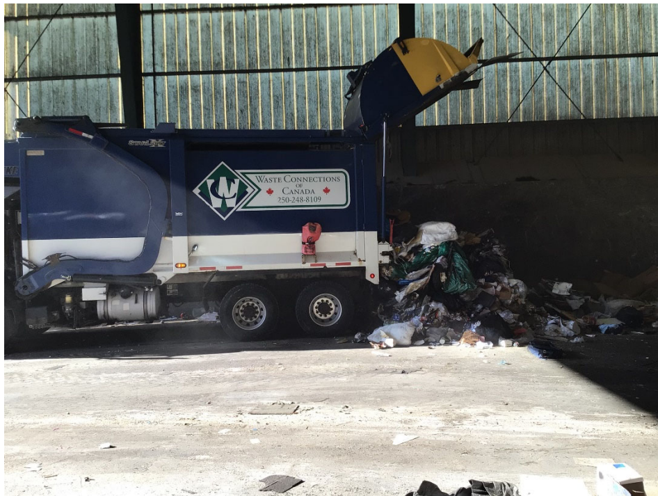
Photo 4: A Garbage Truck Unloading an Industrial, Commercial, and Institutional Load
