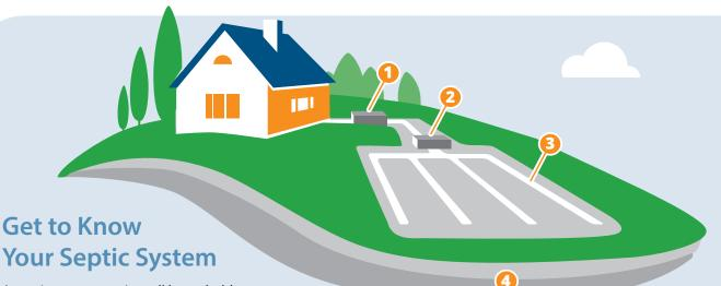
A septic system receives all household wastewater including wastewater from toilets, showers, dishwashers, washing machines, and other plumbing fixtures. Its job is to treat the wastewater so it may safely return to the groundwater and soil.
