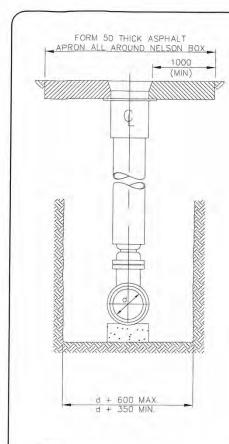
NOTE: JOINT RESTRAINTS AS PER JOINT RESTRAINTS AS PER MANUFACTURER'S RECOMMENDATIONS, ON EACH SIDE OF VALVE. ALL RESTRAINER RODS AND NUTS SHALL BE SUPPLIED BY THE MANUFACTURER OF THE RESTRAINTS USED.
